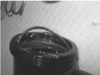
Remove the "O" rings from the body of the valve
