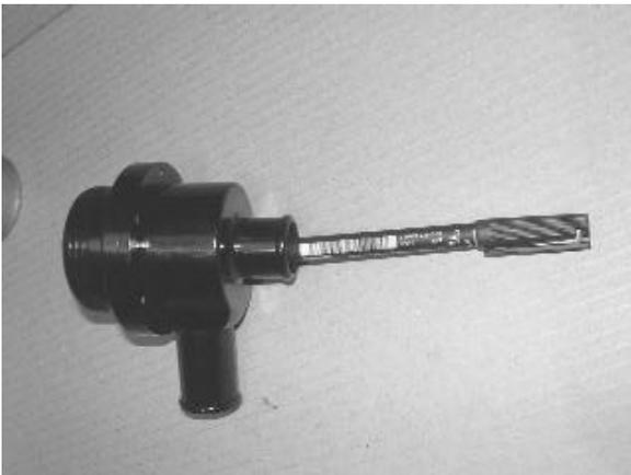
A simple test that you can perform on your valve is to use a pen and push the piston of the valve upwards against the spring to ensure that it moves without restriction. Then with the piston pushed fully up, ie with the spring compressed, place your finger over the top nipple to form a seal.
