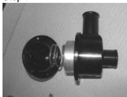
Ensure that the piston moves freely within the body of the valve
