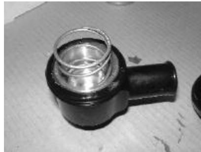
Check that the piston travels freely within the body of the valve before screwing the top back on.
