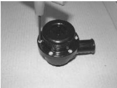
Carefully remove the Allen Cap screws – be aware that the top will spring apart if not restrained
