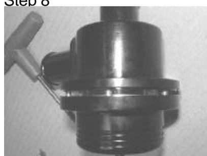
Locate all screws and tighten in a diagonal pattern so that the two parts are drawn together evenly.
