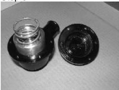
With the top removed you can remove the spring and piston from the valve body and .....
