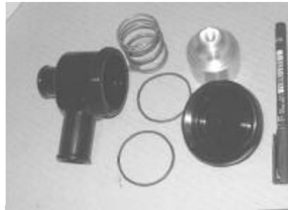
Dis-assembly complete. Carefully clean all the parts with soft tissue or cloth
