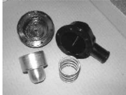
With the dis-assembly completed, wipe all the components clean with a soft tissue or cloth
