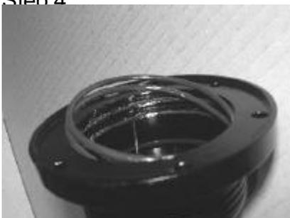
.... Remove the "O" rings from the top of the valve
