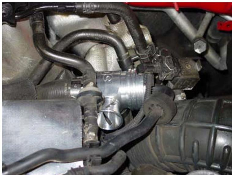
Adjustment of the SPLT-R valve is done by turning the ratcheting adjustment knob located on the top of the valve. Turning the knob clockwise will stiffen the spring for higher levels of boost retention, while turning the knob counter-clockwise will loosen the spring tension for lower levels of boost retention.
