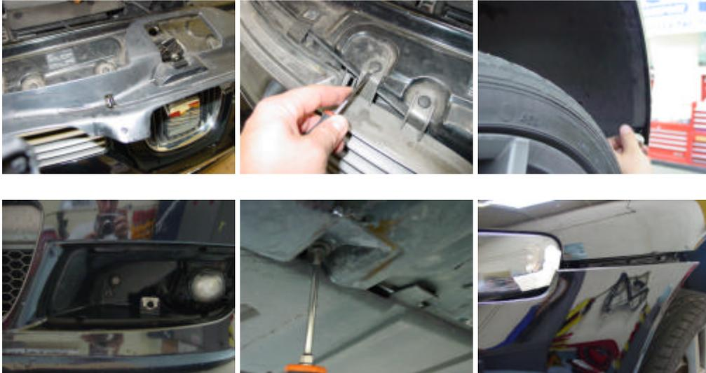
2/ Remove the plastic air ducts from both intercoolers. Remove the left side headlight (4x T30 Torx screws and electrical connections). Loosen the top and bottom hose clips on both intercoolers. Remove the 3x 10mm nuts that retain each intercooler and lift the intercoolers clear. Remove the connecting tube between the intercoolers from inside the engine bay. These have 10mm nuts holding down P clips as per the pictures below.
