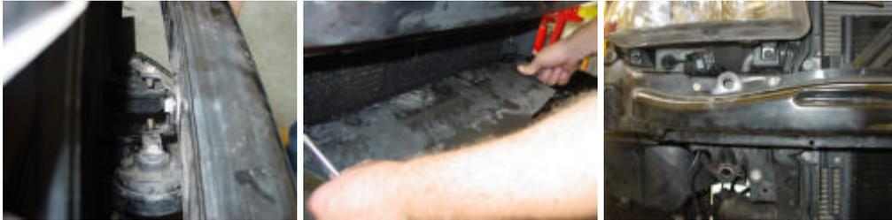
4/ Relocate the horn bracket assembly in to the left front section that has been vacated by the stock intercooler. Fit the horn bracket to the left intercooler top mounting using the top right 10mm nut as per the picture below. Turn the horns so the trumpets are facing downwards to prevent future water ingress. Tidy the wiring using the zip ties supplied.
