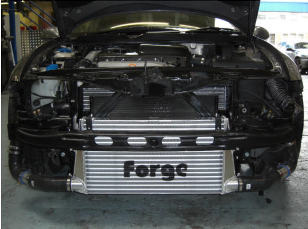
6/ Be sure that all the intercooler mounting bolts, hose clips and the crash bar are secured well. Refit the headlights and refit the complete bumper cover. Remove all tools and lower the vehicle to the ground. You are now ready to enjoy the new performance of your vehicle.
