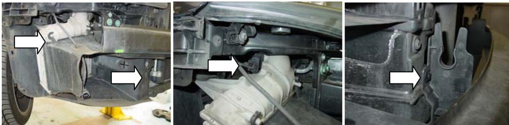
3/ Now remove the front crash bar, this is secured with several 13mm and 10mm bolts.
