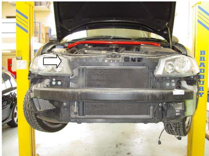
4/ Fit the 2x 300mm silicone tubes to Intercooler inlet and outlet connectors using the hose clips supplied. Fit the aluminium hose joiner to the lower tube as pictured, secure using the hose clip supplied. Mount the new intercooler to the Bumper bar using the cap screws, washers and nuts supplied. Now refit the complete bumper bar and intercooler assembly to the vehicle using the original 13mm and 10mm bolts.
