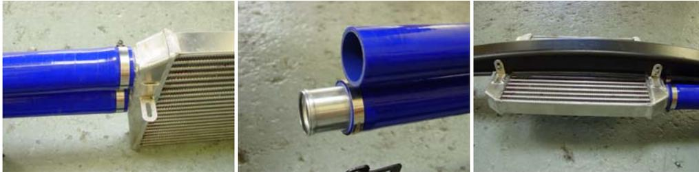
5/ Remove the original Map sensor from the stock intercooler and fit this in to the new aluminium pipe as pictured below. Connect the remainder of the hoses as pictured and secure them all using the hose clips supplied. Check and secure all hose clips that have been fitted to the whole new FMIC pipe run. (If any of these become dislodged at a later stage then it will require the complete bumper removal in order to gain access). Connect the electrical connection to the Map sensor.
