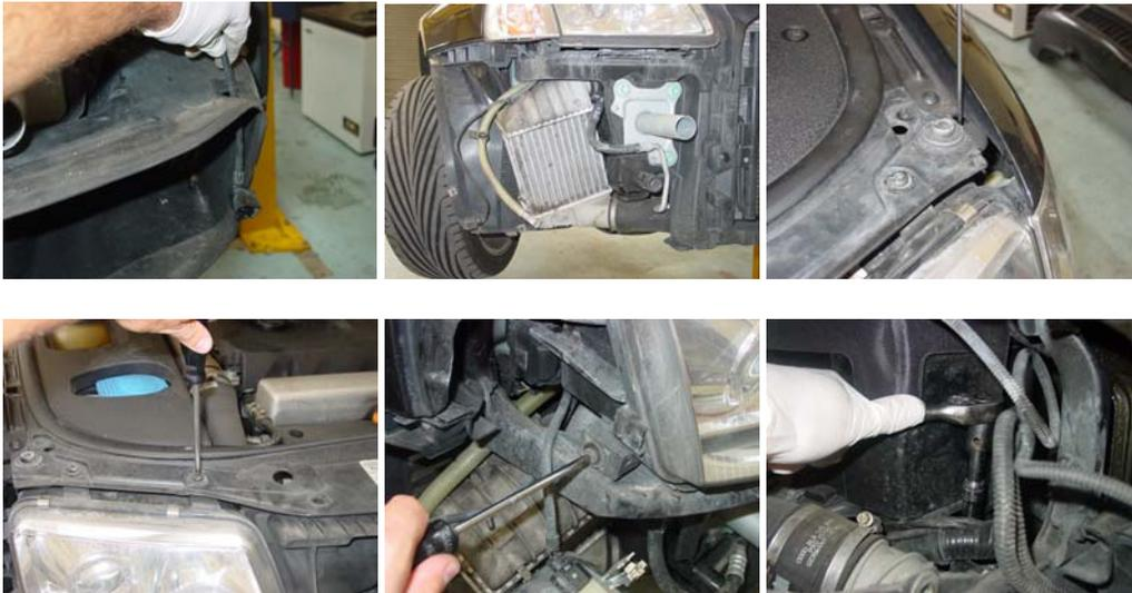
4/ Fit the new intercooler to the new crash bar as supplied using the m6x20 bolts, m6 nuts and penny washers as supplied. Now fit the new crash bar and intercooler assembly to the vehicle using the original bolts nuts and bolts.
