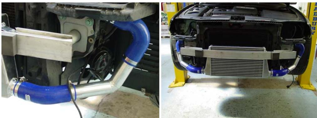
7/ Now refit your bumper as a reverse of step 1. Remember to connect the fog light connectors and also unclamp and connect the headlight washer pipe.
