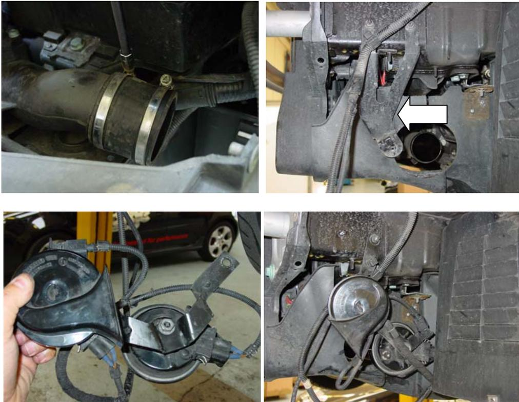
6/ Now fit the 75mm aluminium hose joiners to the upper hoses behind the headlamps on both sides. Fit the 60mm to 51mm reducer silicone hose to this aluminium joiner. Fit the fabricated aluminium pipe to this hose and then use the remaining 51mm 90 degree silicone hose to join to the intercooler. Repeat these steps for both sides of the vehicle. Secure all these connections with the hose clamps supplied. Your installation should look like the picture below.
