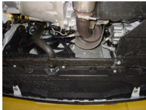
Remove the front sections of both front wheelarch liners by removing the plastic retaining clips. Once the arch liners are loose you can gain access to the 2x10mm bolts each side that retain the bumper to the front wing/fender
