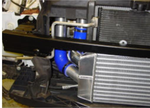
8. Insulate the electrical connection that is now redundant for the original intercooler assistance fan.
