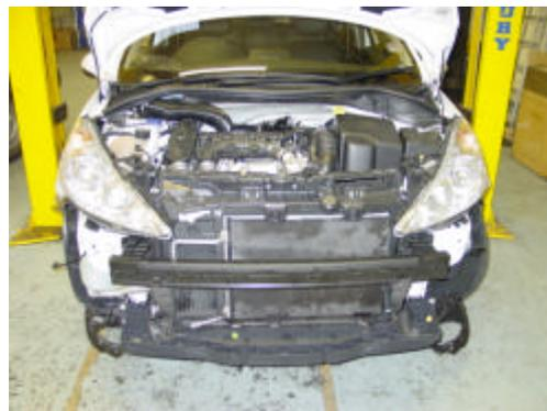
3. Remove the plastic grille on the upper right of the engine bay by turning the 2 slots through 90 degrees to the right. Remove both complete headlamps, these are retained by 3x10mm bolts (two on top, one underneath) and the single electrical connection to each headlight.
