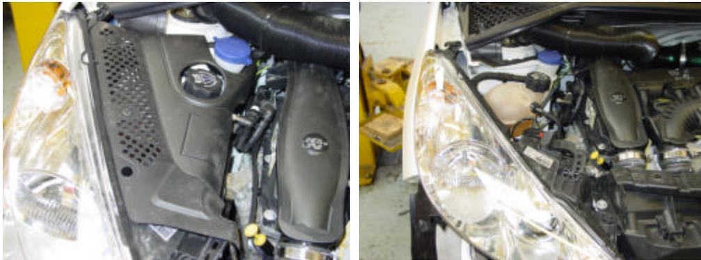
4. Remove the 2x13mm bolts at the top of the radiator panel as shown below. Loosen the two hose clips at the top of the convoluted hoses from the intercooler.
