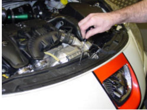
2. Remove the T20 torx screw within each wheelarch. Remove the 2x10mm bolts and the 4 plastic clips that retain the lower edge of the bumper.. Once these are removed, disconnect the fog light connections either side and lift the whole front bumper section clear. See pictures below.
