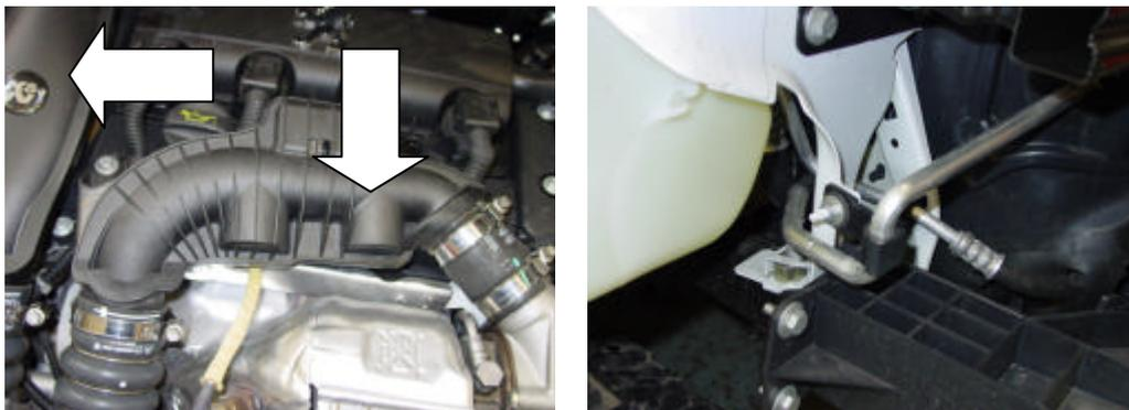
Push the top intercooler retaining clip through the radiator panel so the top edge of the intercooler is free. Disconnect the single electrical connection to the intercooler fan system.
