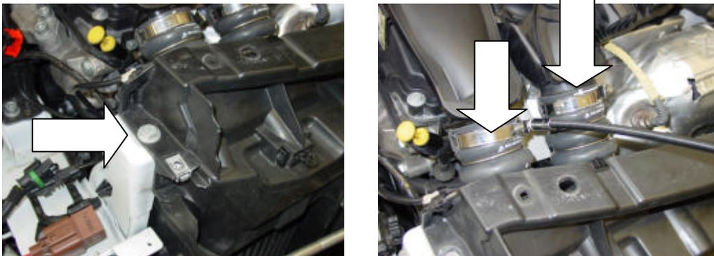
Completely remove the 2 plastic air pipes located on top of the engine (the 2 leading to the intercooler hoses) by removing the 2x10mm bolts that retain each pipe. Remove the single air conditioning pipe bracket on the lower left as you look at the front of the car (see picture below).
