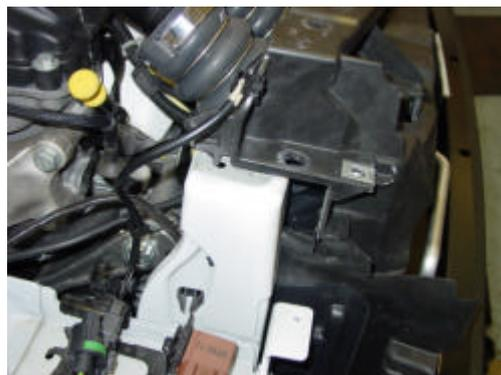
Now lift the intercooler upwards and out from the engine bay (you may need help here to lift both the radiator panel and the intercooler from its location at the same time) Be careful not to damage the small bore water overflow pipes that run just behind the intercooler.
