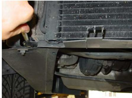
4/ Remove the plastic intake ducting from the stock Intercooler. Remove the outer hose completely by removing the 2 hose clips as pictured. Remove the 3x 10mm headed bolts that retain the stock intercooler. Lower the intercooler down and remove the hose clip on the upper pipe connector, then remove intercooler completely from the vehicle.
