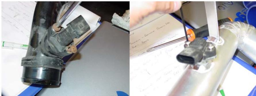
9/ Secure the new Front mount Intercooler using the bolts and washers supplied as per the picture below. Do not fully tighten the bolts until the whole assembly is fitted in to place.
