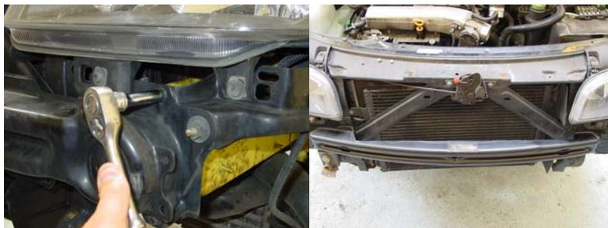
3/ Remove the 3x 10mm nuts/bolts that retain the radiator undertray and remove the undertray completely.
