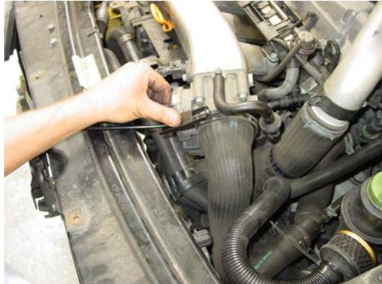
8/ Remove the MAP sensor from the original plastic pipe and fit to the new aluminium pipe as pictured. Use the 2x "m5x16" new cap head screws to secure the MAP sensor to the new pipe.
