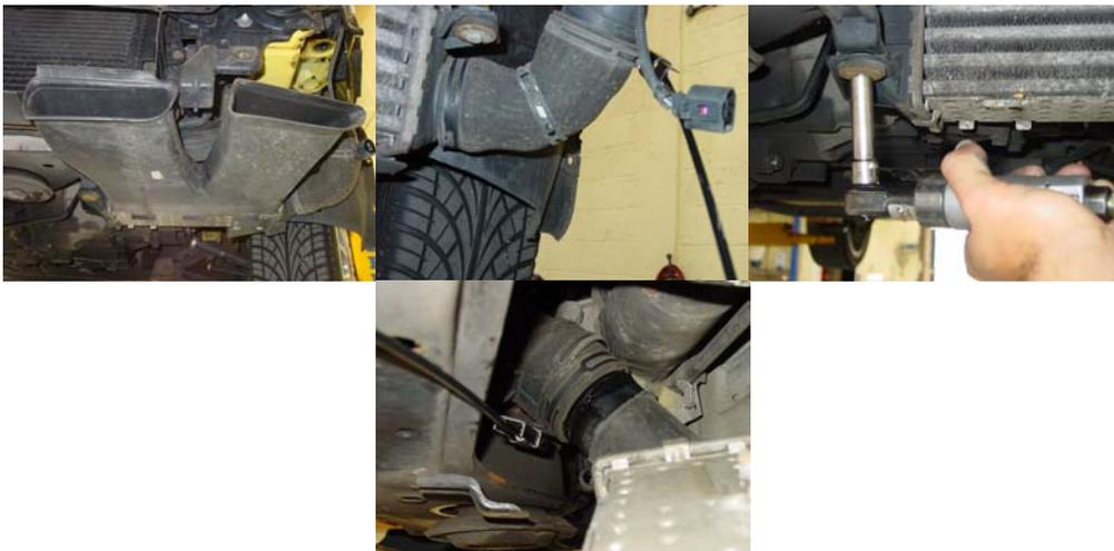
5/ With the intercooler now out of its location it is possible to remove the remaining plastic and rubber pipe that joins the intercooler to the upper aluminium boost pipe as pictured below. It may be necessary to remove the engine cover to gain access to these hose clips. Remove all parts indicated by the arrows but leave the aluminium pipe in place.
