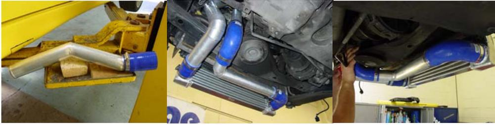
13/ Remove both honeycomb grilles from the lower inside section of the front bumper. Then trim all the plastic fixing lugs so they are flush with the edges of the intake air ducts as shown below. It may also be necessary to trim the inner lower edge of the front bumper to sit around the new intercooler without distorting the plastic intake slats. You will only know how much (if any) trimming is required once the refit of the front bumper takes place.
