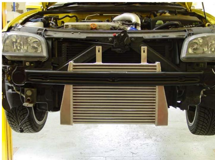
10/ Cut then original intercooler bracket as per the picture below using a hacksaw or small grinding tool. Only remove completely if you are 100% sure that the stock intercooler will never require refitting.
