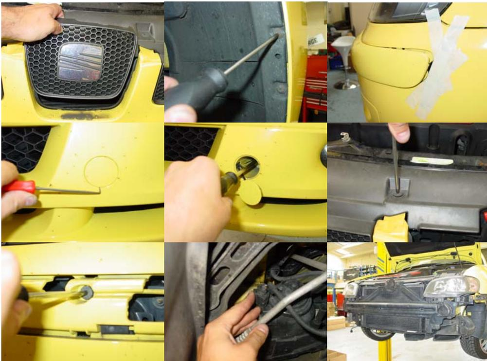
2/ Remove the 4x 8mm headed bolts and the 4x 13mm headed bolts from the steel crash bar and remove the complete unit. Fit the new supplied bumper bar in to the same place using the existing bolts and washers.
