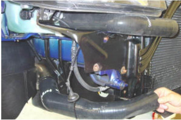
Install the lower intercooler hose as shown
