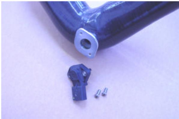
If your original intercooler had a MAP sensor installed, refit the sensor to the new hose. If no sensor was present, use the supplied blanking plate to seal the sensor housing in the new hose
