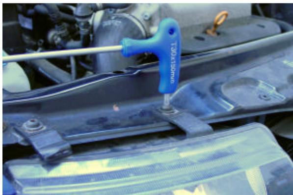
Remove the two upper and two lower torx bolts from the headlight unit on the intercooler side of the vehicle. Disconnect the electrical connector and remove the headlight unit.
