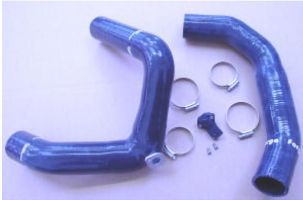
Identify the two new hoses supplied with this kit. One of the hoses has an alloy insert bonded into the hose – this will be the upper hose.
