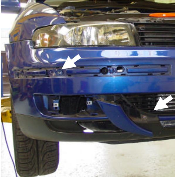
On the front of the plastic over bumper, remove the two black plastic rubbers using a bladed screw driver and then remove the Torx bolts.
