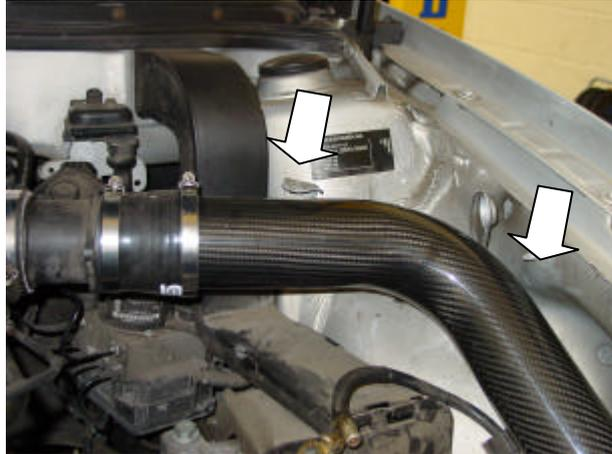
8/ If your original air box had the secondary air feed in to the side then fit the air breather filter and adapter as shown below, use the hose clips supplied. Make sure the hose does not hang down too low and foul the gear linkages on top of the gearbox.
