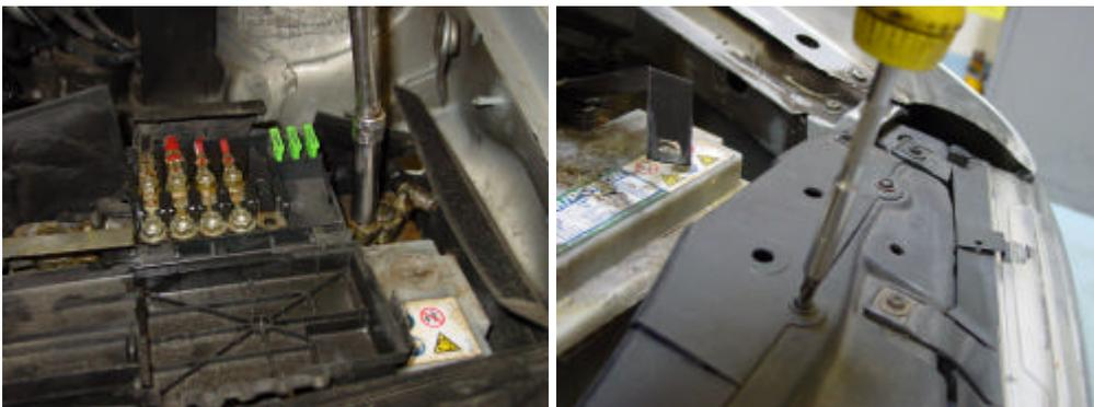
3/ Remove the complete left side headlight, firstly disconnect the electrical connection and then the 4x T30 screws.
