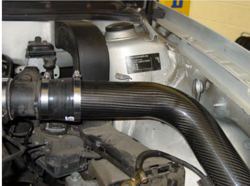
6/ Now fit the silicon hose to the end of the carbon pipe as shown, then the aluminium 40 degree joiner and the filter in turn as shown below. It may be necessary to protect the 40 degree aluminium joiner from the surrounding bodywork, do this by fitting the split tubing as indicated to any sharp edges. Make sure all hose clips and fittings are secure.
