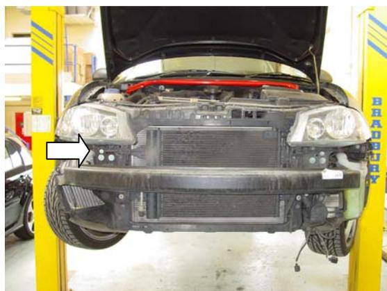
5/ Fit the 2x 300mm silicone tubes to Intercooler inlet and outlet connectors using the hose clips supplied. Fit the aluminium hose joiner to the lower tube as pictured, secure using the hose clip supplied. Mount the new intercooler to the Bumper bar using the cap screws, washers and nuts supplied. Now refit the complete bumper bar and intercooler assembly to the vehicle using the original 13mm and 10mm bolts.
