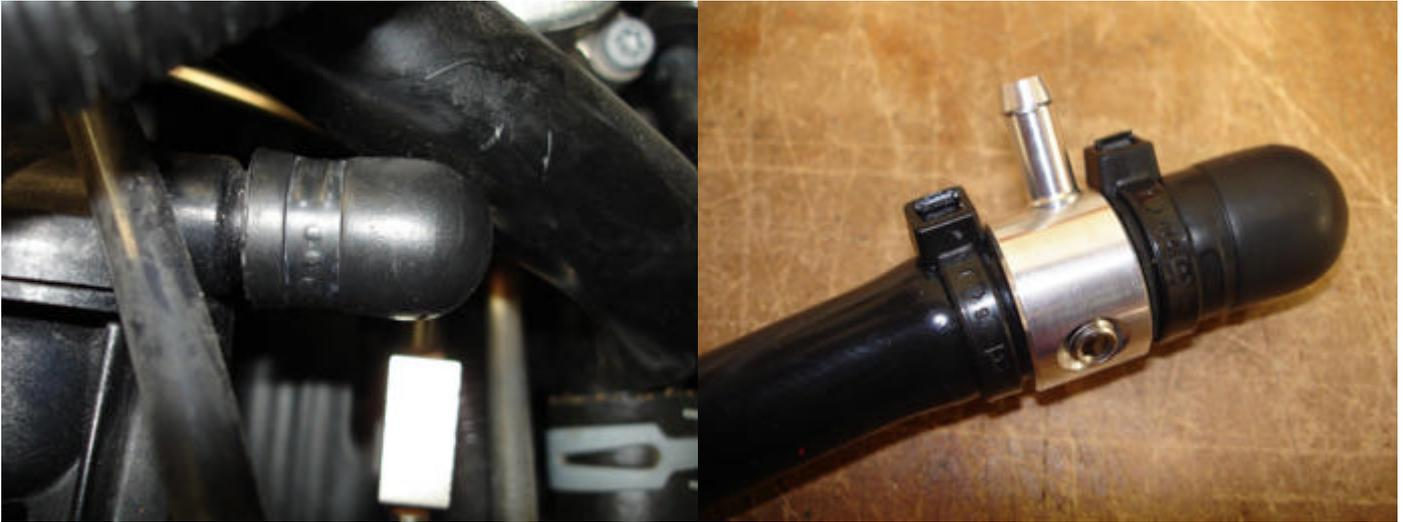
This installation will be identical to that of a transverse engine application except that one end of the vacuum tap is capped off instead of connected to a check valve with another piece of vacuum hose.
