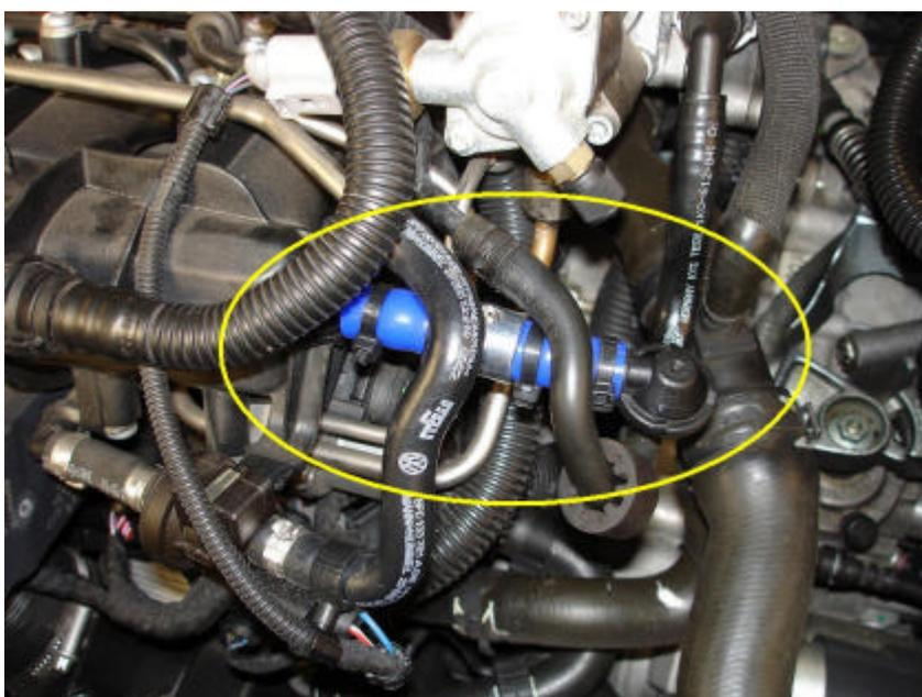
On a longitudinal engine application, specifically just the B7 chassis Audi A4, you will need to find the rubber blanking cap located on the intake manifold at the back side of the motor close to the firewall. Remove the single one time use clamp securing it, and remove the cap as well, saving it to be swapped onto the end of the vacuum tap as shown below.
