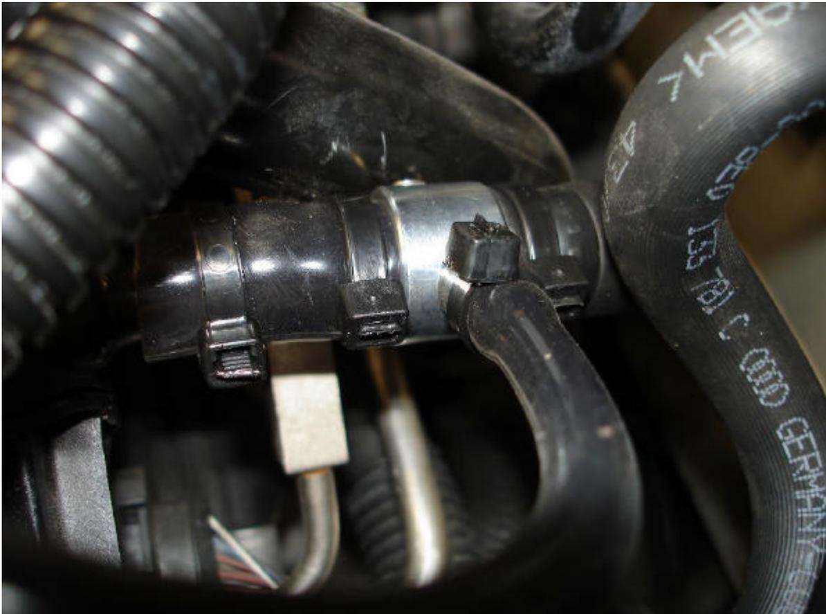
From the appropriate nipple on the vacuum block (largest port), run a length of vacuum tubing along the top of the motor, around the passenger side, down to the remaining linear port on the solenoid you mounted previously. (See plumbing diagram) Secure both ends of this line using two of the included zip ties. Use additional ports on the vacuum tap as needed.
