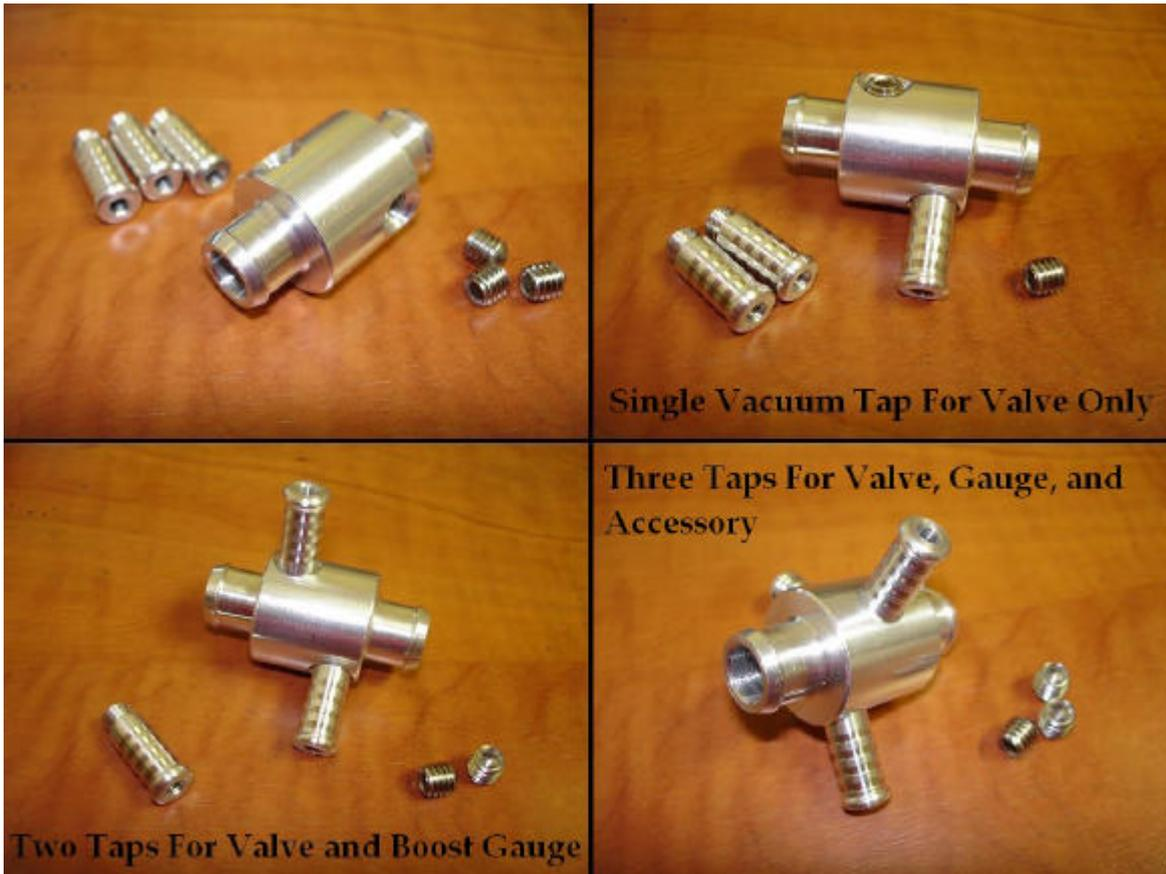
To install the vacuum tap, you must first remove the engine cover. On all transverse engine applications, MK5, B6 Passat, Eos, Audi A3, TT, etc., remove the two OEM one-time use clamps from the small hose connecting the small 3-way check valve to the side of the intake manifold. You may choose to save this length of OEM hose for possibly returning the car to stock later.
