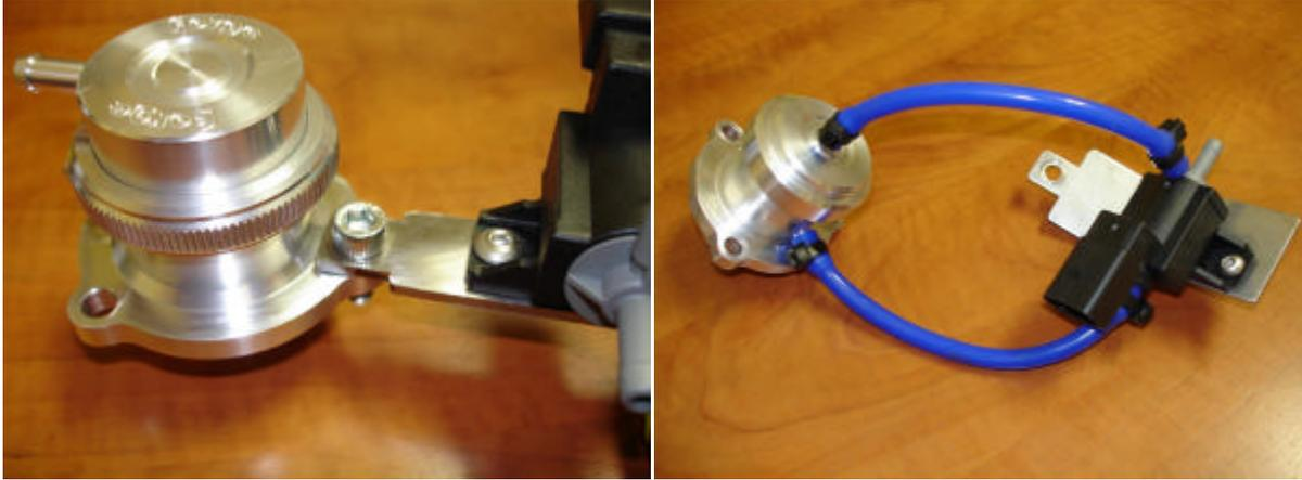
With the new Forge valve loosely mounted to the turbo, and a location selected for the solenoid and it loosely mounted as well, you will now measure to find the appropriate lengths for the vacuum hose connections between the valve and the solenoid.
