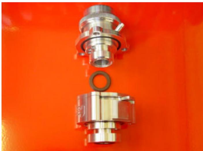
Also, when installing the larger stepped o-ring into the base of the valve for use with the adjustable valve spacer, please apply a small amount of the supplied synthetic bearing grease to the bottom of the o-ring prior to inserting the valve into the adjustable spacer for installation. This will aid in allowing smooth adjustments of the spacer without removal of the valve from the car to make adjustments.
