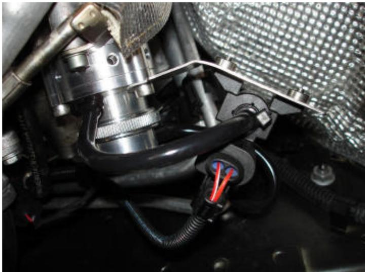
As mentioned above, for the purpose of generating these instructions, we will be mounting the solenoid bracket using one of the bolt holes for the new Forge valve. The mounting hole of the solenoid bracket can be placed over a mounting hole on the valve itself (positioned away from all other parts within the engine bay) and an OEM valve bolt can be used to secure the solenoid bracket on top of the Forge valve mounting hole.
