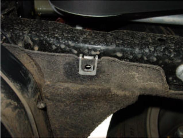
At the front of the vehicle, where the plastic cover was removed, there is a fastener attached to the wheel arch lining material that requires removal so that it can be re-used.
