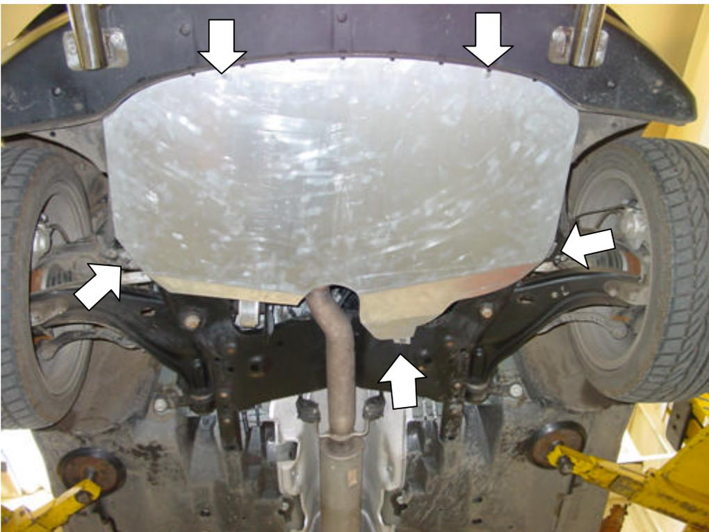
The undertray can now be lifted into position and secured with the fasteners. Rotate the fastener screws  $\frac{1}{4}$  turn clockwise to lock.
