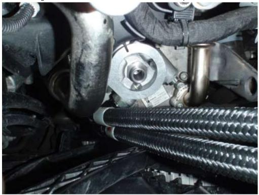
4. Feed the braded hoses through the radiator pack as shown below screw on the NA dash fittings and tighten. Please refer back to the intercooler instructions to replace bumper.
