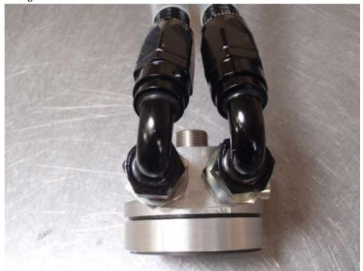
3. Place the spacer plate assembly were the oil filter screws on, Tighten in position shown below making sure there is clearance all around and then replace oil filter.
