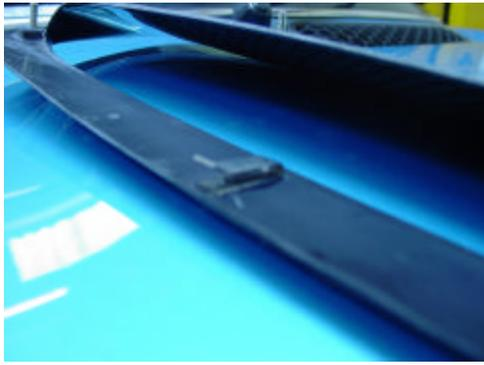
Note - the replacement scoop has a retaining clip on the rear edge.
