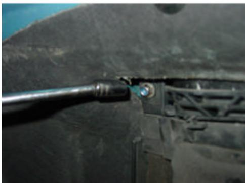
The external scoop should be aligned to ensure that it is evenly located within the recess before the securing nuts are tightened from the underside.
