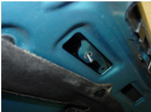
The internal plastic air duct is then refitted and the supplied washers and nuts installed - but left loose at this stage.
