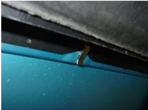
This clip is slotted over the rear metal work by offering the new scoop to the hood / bonnet at an angle at first. The scoop securing studs are then allowed to pass through the hood / bonnet fixing holes
