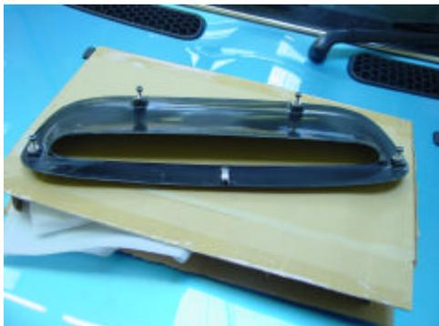
The replacement scoop as supplied will have the fixing nuts and washers in place. These will need removing prior to install
