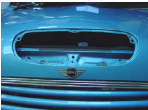
With the original scoop removed completely the new scoop can be installed.
