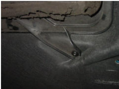
After raising the hood / bonnet of the vehicle, remove the intercooler air duct which is secured at the rear by two cross point screws and at the front by the external bonnet / hood scoop fixing bolts. It is a good practice and as a safety precaution, subject to the vehicle engine being cold to first drape an old sheet or cloth across the engine bay so that if any parts are dropped by accident they are easily recovered.
