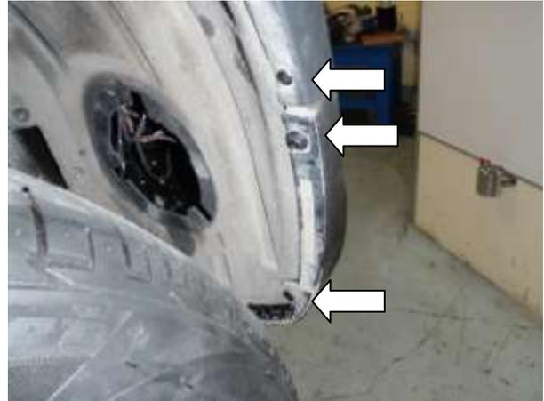
1. Park vehicle securely, jack the front of car and support on axle stands so that the front wheels are clear of the ground and raise bonnet. Starting on the driver's side turn steering wheel so the wheels are on full lock to gain access to the arch liner. Undo the 8mm screw, push out the pins from the three pin clips above using 2mm pin punch, then pull out the center of push clip using the flat bladed screw driver. Repeat this on the passenger side.
