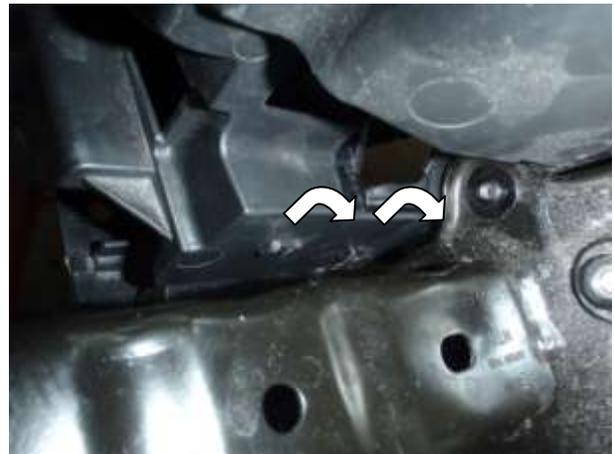
8. There are two plastic ducts which need to be removed to gain access to the stock intercooler. At the top of the ducting push the clip on the side inwards, and push the ducting down and out. To release the bottom, lift the ducting up and out to release the bottom clips.
