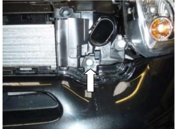
7. Remove the two T25 screws as indicated above and the bumper is now free to remove.
