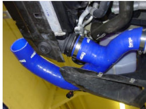
**7/ Fit the 2x plastic expanding nuts in to the square holes in the lower radiator panel. Screw on the brackets with the new screws supplied.**
