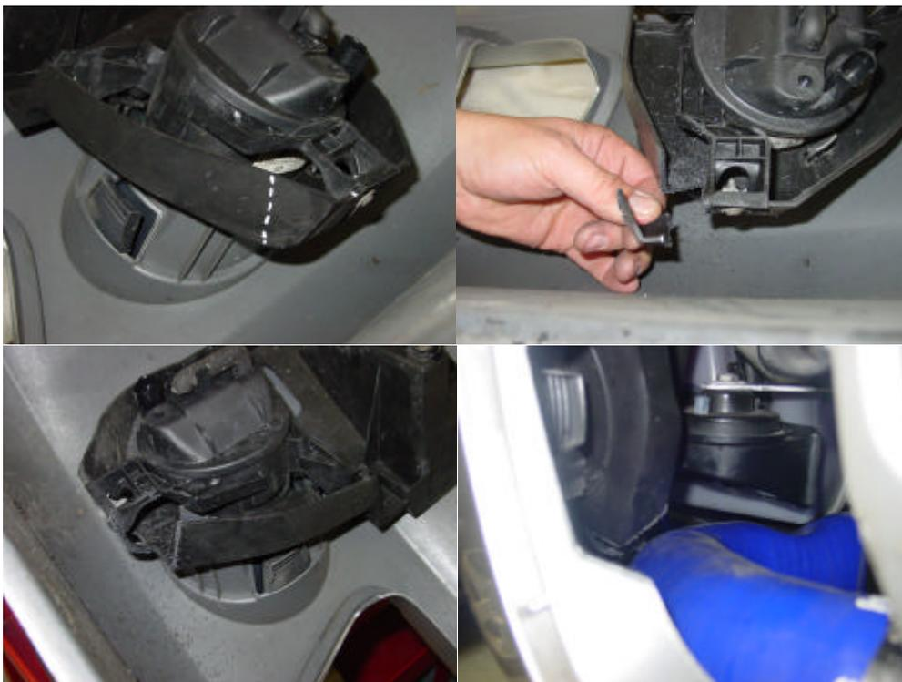
**10/ Refit the complete front bumper making sure of fog light clearance on the hoses. Remember to reconnect the fog lights and air temp sensor. Refit the engine under tray. Clear away all tools and close bonnet.**
