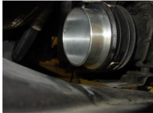
**6/ Fit the new hoses as pictured below. Use the hose clips supplied but do not tighten at this stage.**
