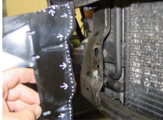
**3/ Remove the complete engine under tray. This has 8x T25, 1x T30 and 2x 5mm Allen bolts securing it to the underside of the car.**
