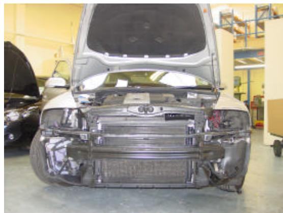
**2/ With a disc cutter or hacksaw remove the metal deflectors as pictured below.**
