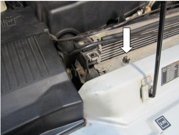
Remove the plastic pipe from the two clips and move out of the way.
