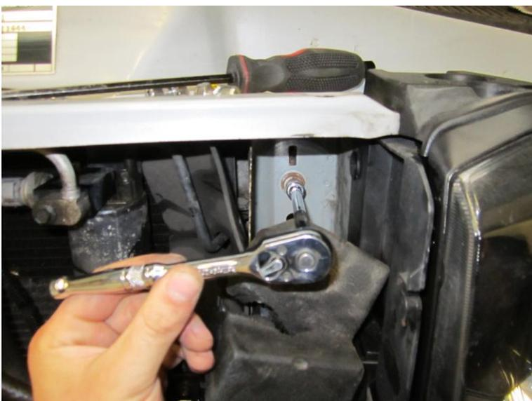
Undo the 10mm bolt and remove the bracket behind the slam panel.
