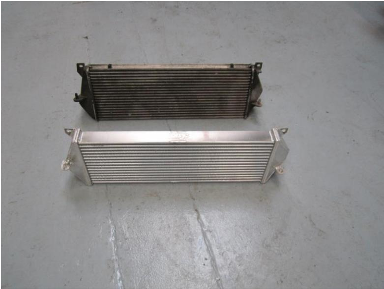
Pull the intercooler out, you will need to lift the passenger side out first (RHD car)
