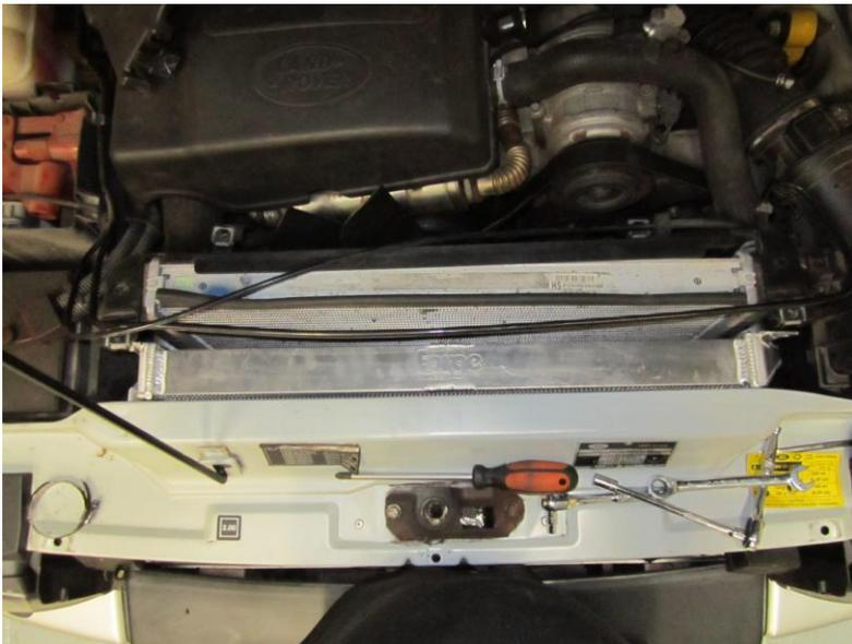
Fit the Forge intercooler again you will need to lower the driver's side in first (RHD car).
