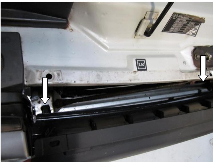
Pull the Grille towards you then pull upwards to release the grille from the vehicle.
