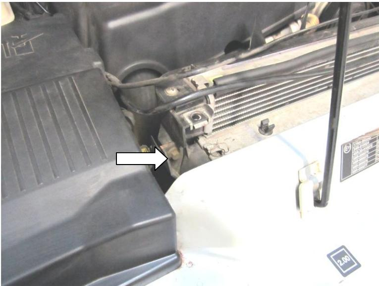
Undo the 10mm intercooler to radiator bolt
