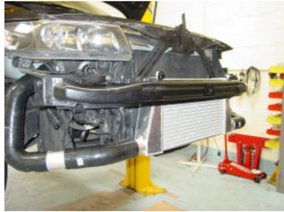
6/ Be sure that all the intercooler mounting bolts, hose clips and the crash bar are secured well. Refit the left hand headlight and refit the complete bumper cover. Remove all tools and lower the vehicle to the ground. You are now ready to enjoy the new performance of your vehicle.
