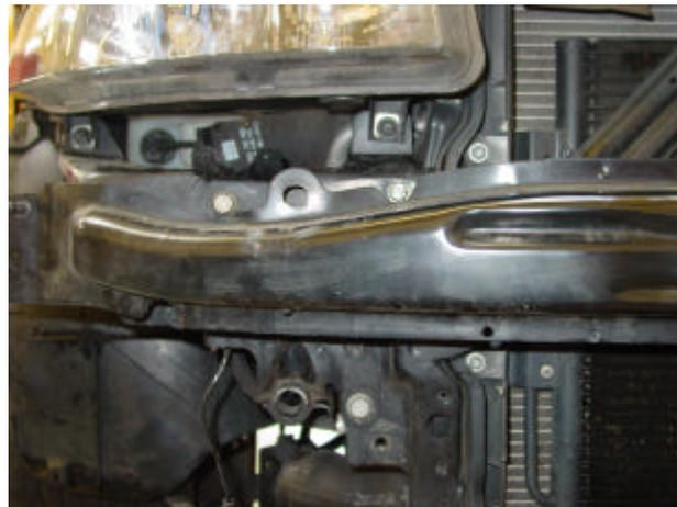
4/ Relocate the horn bracket assembly in to the left front section that has been vacated by the stock intercooler. Fit the horn bracket to the left intercooler top mounting using the top right 10mm nut as per the picture below. Turn the horns so the trumpets are facing downwards to prevent future water ingress. Tidy the wiring using the zip ties supplied.
