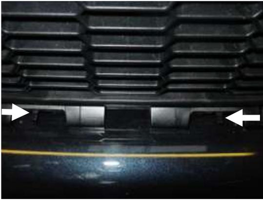
At the base edge of the grille there are four levers. When pushed towards the centre of the vehicle they allow the release of the grill from the bumper cover.
