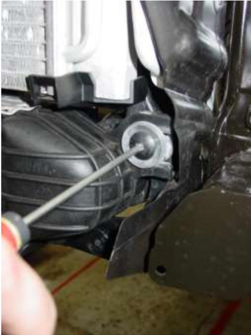
The Original intercooler mounting screws (T25 Torx) can now be removed from each side of the intercooler.
