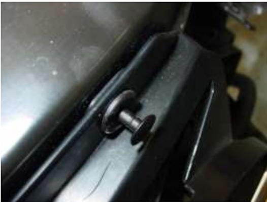
Firstly the vehicle will need to be secure and raised to allow the removal of the front wheels. The hood or bonnet of the vehicle should be opened. The grill needs to be removed. This is secured at the top edge by four plastic fasteners (push pins). The center pin of the fastener is prized out with the blade of a flat screw driver. This allows the fastener to be withdrawn from its locating hole.
