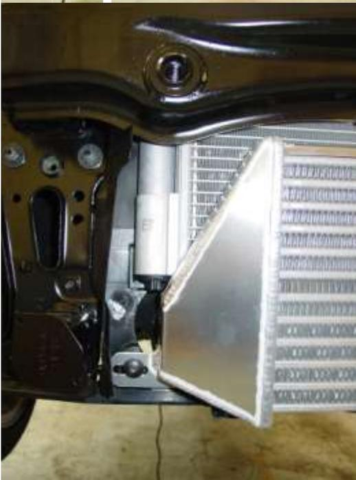
In the centre at the top of the new intercooler there is a bracket that will secure the intercooler to the metal crash bumper. In order to attach this, a 6.5 mm or 1/4" hole requires drilling. To facilitate this, with the intercooler in place, mark the required position of the hole on the crash bumper.
