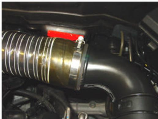
The flexible intake hose of the induction kit is fitted the cold air feed (hard plastic pipe and secured with a hose clamp).
