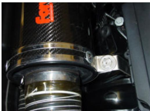
The carbon canister / filter housing is secured to the previously fitted bracket with the M8 x 25mm hex bolt and Nyloc nut. A washer is used between the bolt head and the canister bracket as shown.
