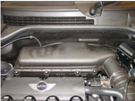
At the rear of the engine the Air Box is located.
