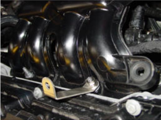
The bracket that will secure the new induction kit is fixed to the intake manifold stud using the 13mm locknut.
