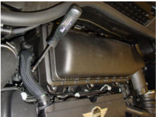
Remove the T25 Torx screw that secures the airbox
