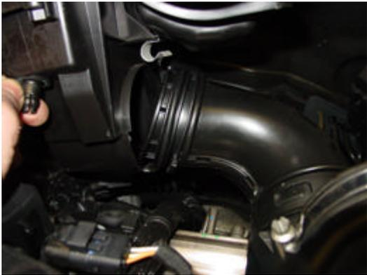
The intake air feed pipe clips into the side of the air box and can now be pulled free.
