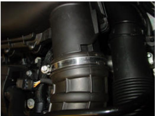
Loosen the hose clamp that connects the intake hose to the air box and pull the hose off.
