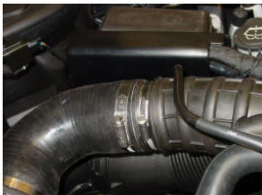
The induction silicone elbow from the induction kit is connected to the rubber intake hose with the alloy hose joiner and secured with the hose clamps.
