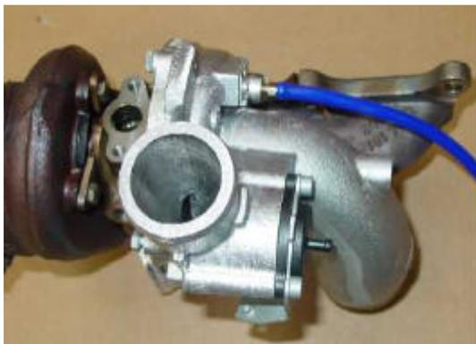
Identify the hose that connects to the turbo compressor housing
