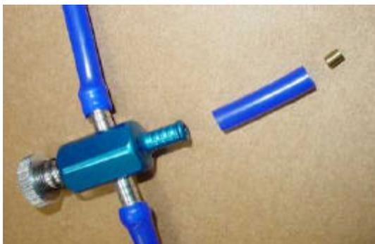
The (BV) or (ICBA) may need a small brass restrictor installing into a short hose connected to the base of the valve or a restrictive nipple connector. These are optional and should be specified when ordering. If either of these have been specified, then in order to increase maximum boost the restrictor can be drilled out.
