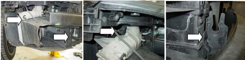
3/ Remove the right side headlight completely, this is fixed with T35 torx screws, also disconnect the electrical connections in order to remove the complete headlight unit. Remove the lower rubber boost pipe which connects to the hard pipe in the lower engine bay as indicated below.
