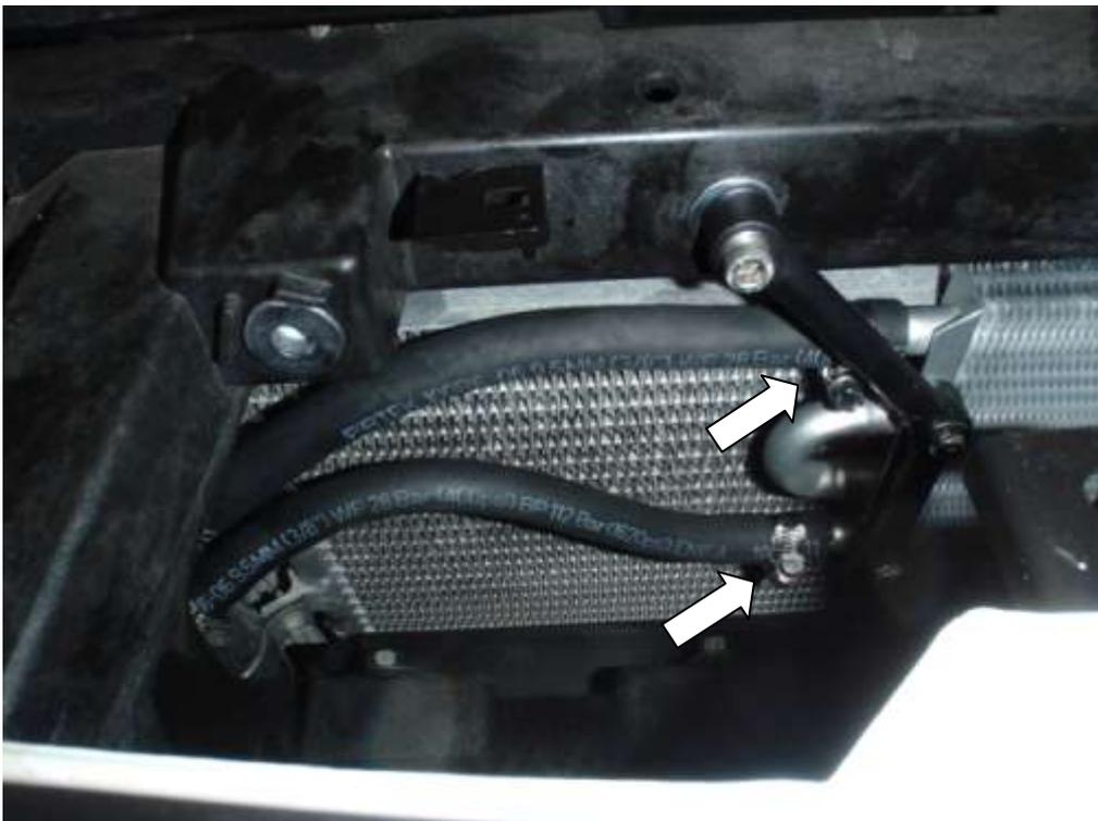
10. Installation is now complete. Replace the slam panel, remove hose clamp from step one top up the PAS tank. Bleed your system buy turning the steering wheel, small increments at first leading up to full opposite lock.
