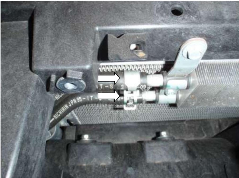
5. Undo the 10mm bolts holding the PAS oil cooler in position and remove.
