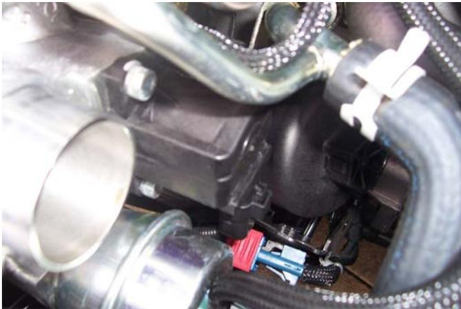
**4)** We would recommend moving the radiator fluid tank to further gain access to the solenoid. It can be easily moved by undoing the one 8mm screw.
