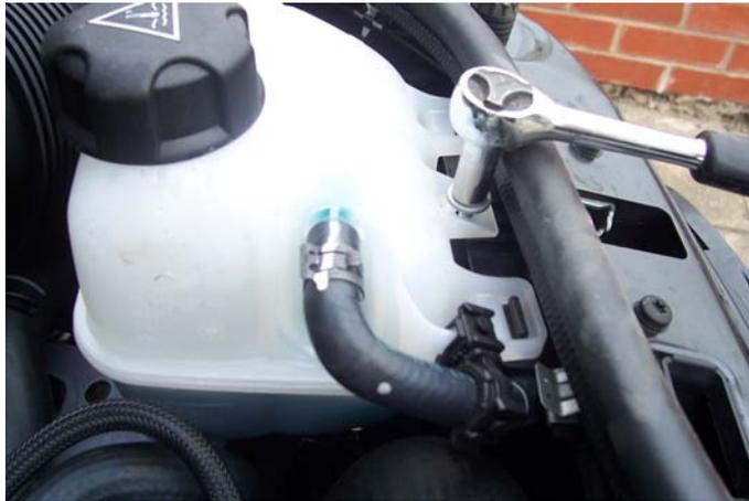
**5)** Next, remove the 3 bolts on the original solenoid using an Allen key (access is restricted at this point and it is recommended to check access to all bolts before proceeding)
