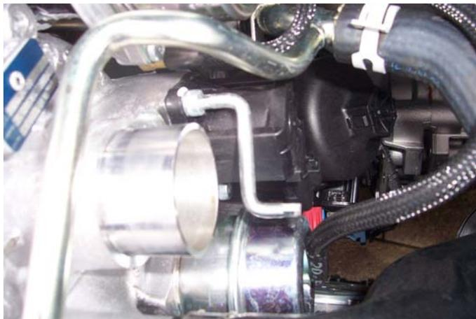
**6)** Once the solenoid is removed carefully place it to one side or disconnect from the loom and remove from the vehicle. You can now offer up the blow-off adapter (placing the forge logo at the lowest side). \* Do not insert bolts at this time.
