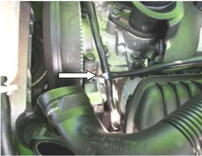
Cut the original rubber vacuum hose in the shown location
