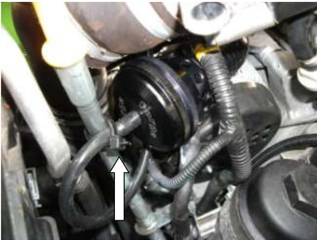
Fit the Dump valve into the silicone T piece and secure using the supplied 35mm hose clamp.
