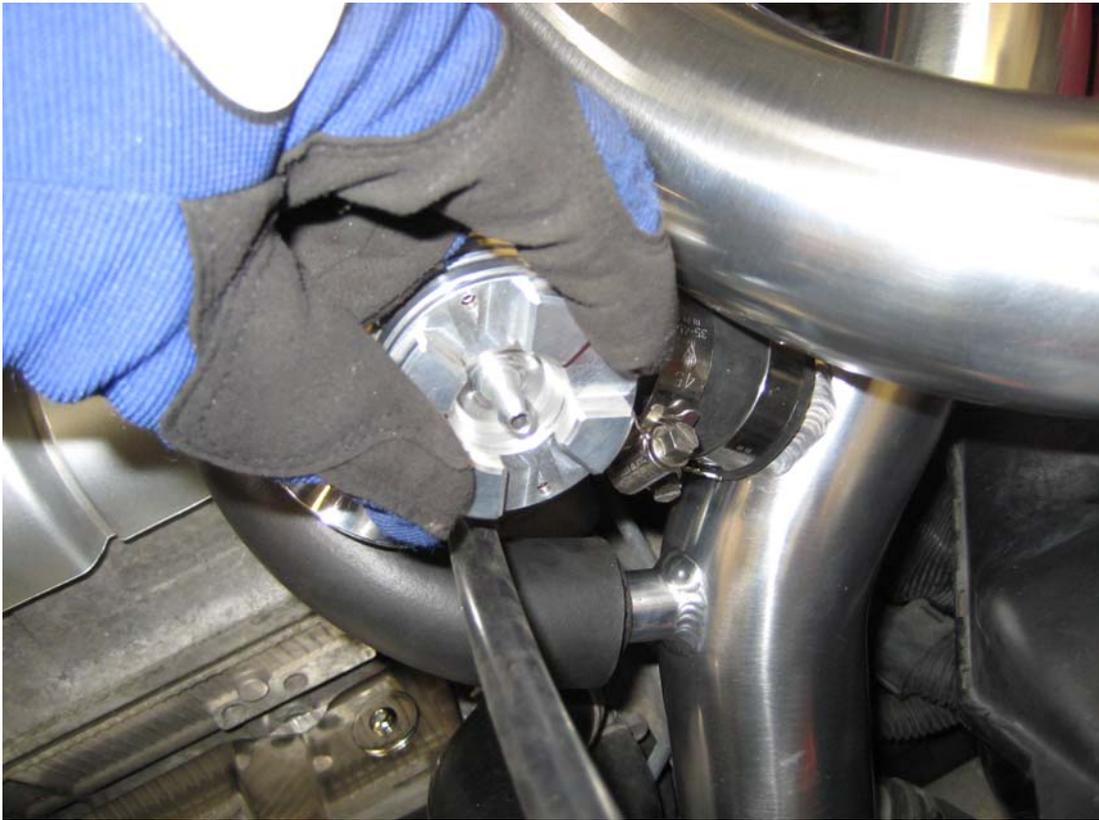
10. Connect the vacuum line to the top of the valve and put the spring clamp back in place to hold the line on the dump valve. Start the engine.
