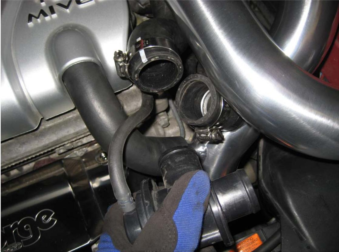
4. ....then locate where the vacuum line joins the engine, and squeeze the spring clamp with your needle nose pliers to loosen it, and pull it back down the vacuum line.
