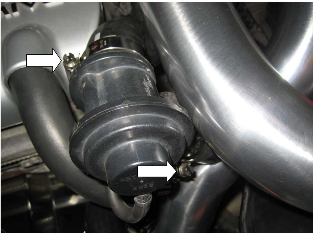
3. Pull the inlet and outlet hoses from the valve, and release the valve from the pipes.....
