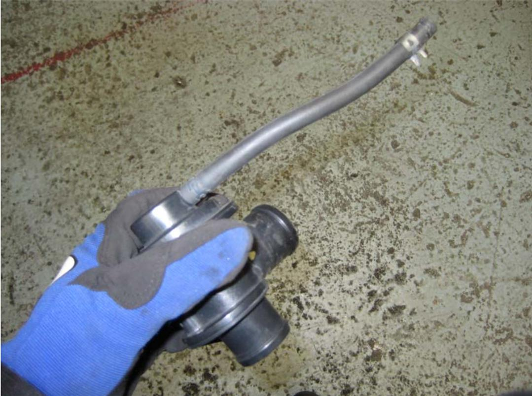
6. Remove the spring clamps from the vacuum line and place them onto the new silicon vacuum line supplied, about 50mm from the ends. Push the new vacuum line onto the port on the engine, and secure it with the spring clamp. Leave the other end disconnected at the moment.
