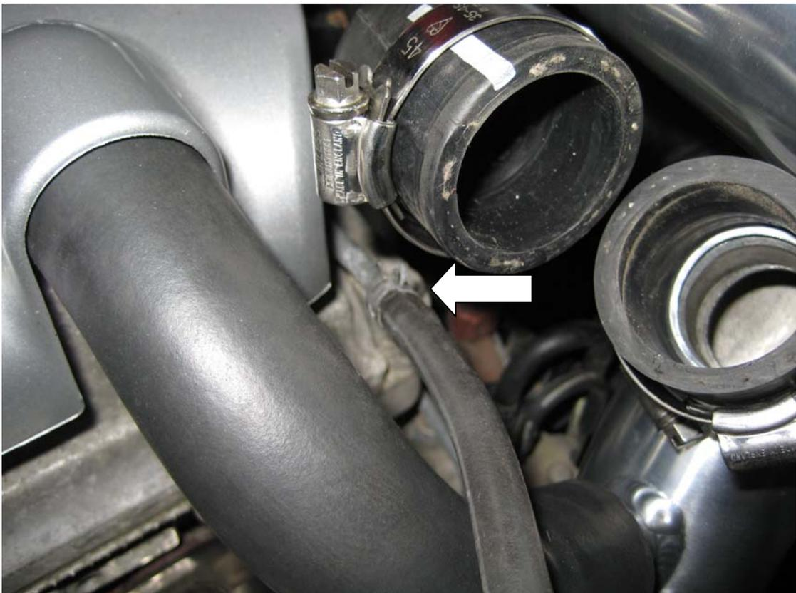
5. Remove the valve with the vacuum line attached from the car.
