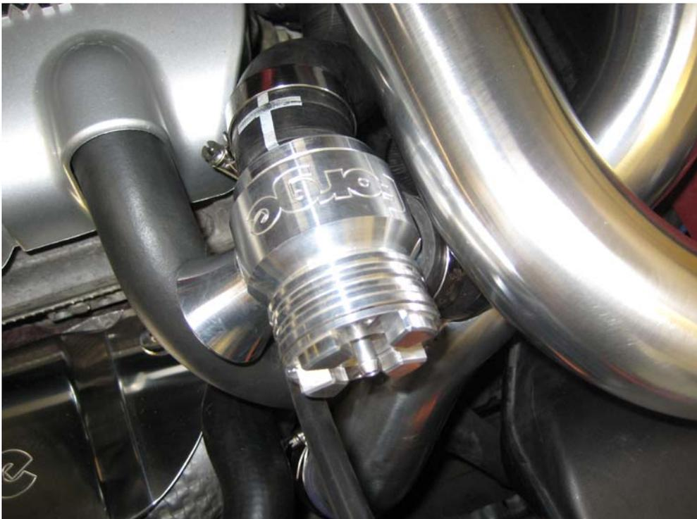
9. You now need to adjust the tension on the spring – the Split-R is fitted with a conical spring which can be adjusted to suit the boost you are running. Adjustment is made by turning the castellated top part of the valve either clockwise to INCREASE the tension or anticlockwise to DECREASE the tension. The adjuster is ratcheted so as it's turned it will 'click'.
