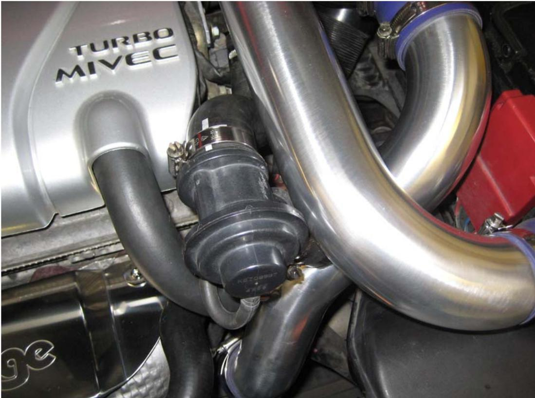
2. Loosen the two retaining hose clamps with either a 7mm or 8mm hose clamp driver, screwdriver or socket.
