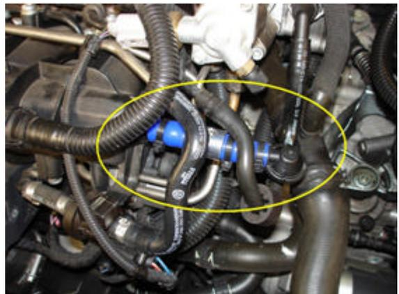
To install the vacuum tap, you must first remove the engine cover. On all transverse engine applications, MK5, B6 Passat, Audi A3, TT, etc., remove the two OEM one-time use clamps from the small hose connecting the small 3-way check valve to the side of the intake manifold. You may choose to save this length of OEM hose for possibly returning the car to stock later.
