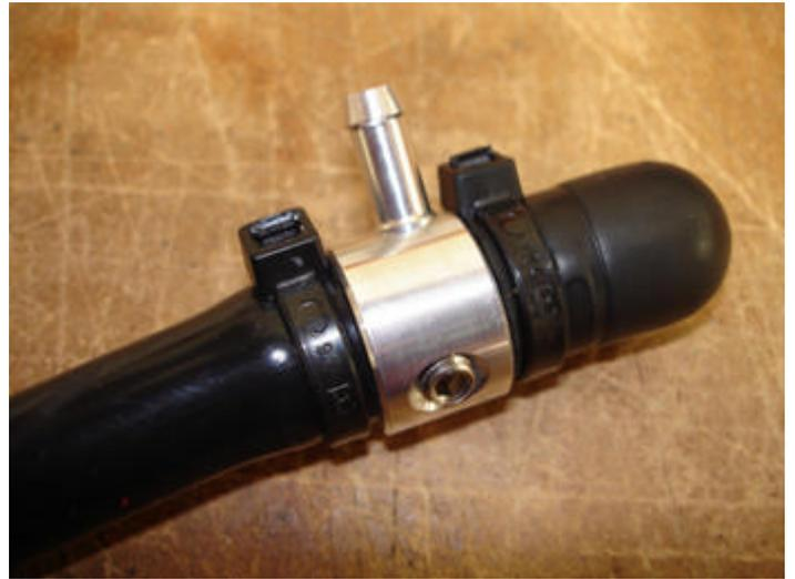
This installation will be identical to that of a transverse engine application except that one end of the vacuum tap is capped off instead of connected to a check valve with another piece of vacuum hose.
