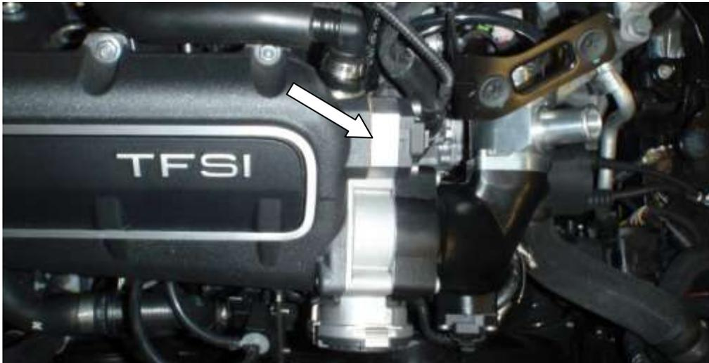
8. Forge highly recommend venting to atmosphere as this valve has a bigger bore for releasing the boost pressure. However you can install this valve recirculating if you wish. Follow step one in reverse order and your installation is now complete.
