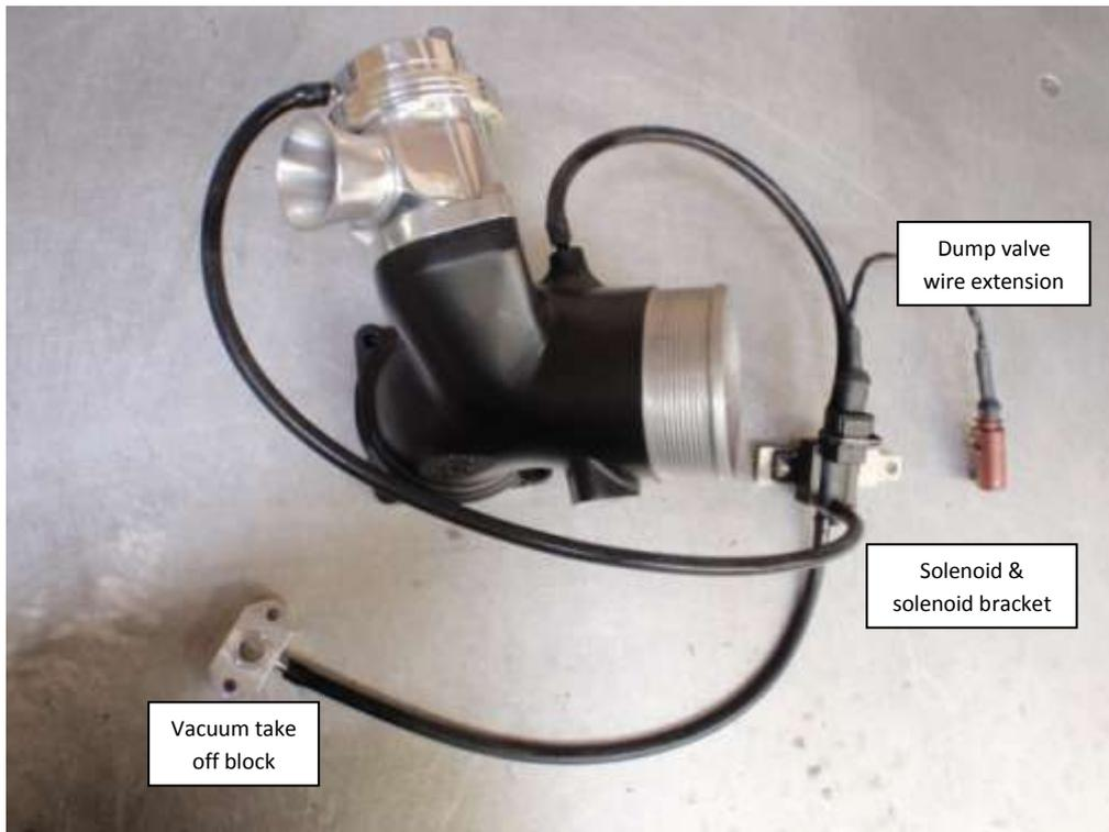
6. If there are any clearance issues when the high flow inlet and dump valve is fitted. Remove the dump valve with a 5mm allen key, on the base of the flange you will see two small bolts undo with a 3mm allen key. Rotate to the appropriate position and reattach dump valve. Push the dump valve plug under the oil filler cover bracket and wires .Connect to the solonoid by plugging into the wiring extension.
