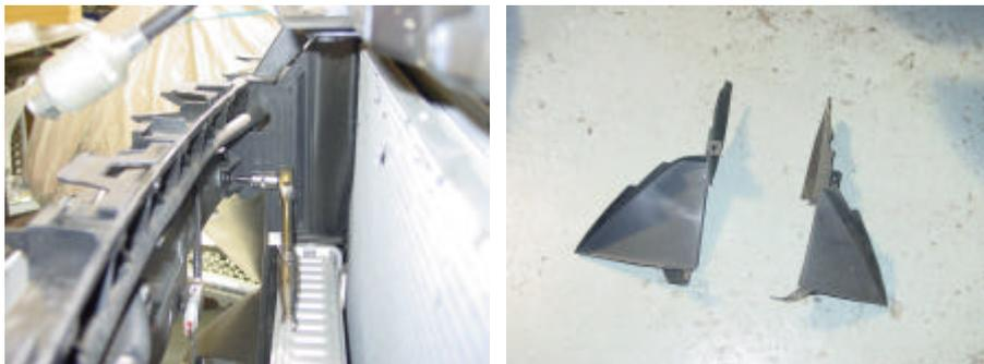
**3/ Loosen the 2 lower hose clips from the original intercooler pipe connections. Remove the 2x 8mm bolts from the intercooler lower fixings. Now lift the intercooler slightly in order to remove it from its upper mountings and then ease forwards whilst removing the 2 hose joints. Completely lift original intercooler away from the vehicle.**
