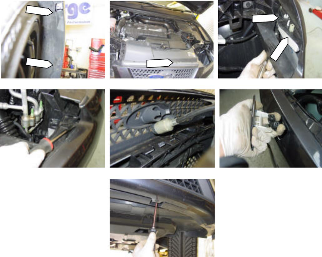
**2/ Remove the 2 plastic air guides. These are fixed with a single T30 screw on each side. These will not be refitted later due to the new larger intercooler fitment.**
