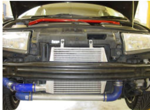
19/ Fit the longest length of aluminium tube as per the left picture below and the remaining 45 degree silicone hose to the other end pointing toward the original lower pipework.
