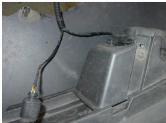
8/ Remove the air guide that is clipped to the outside of the intercooler.
