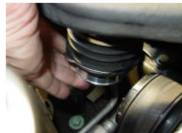
17/ Fit the 45 degree silicone hose to the intake pipe as pictured below. Use 2 x hose clips provided but do not tighten at this stage.
