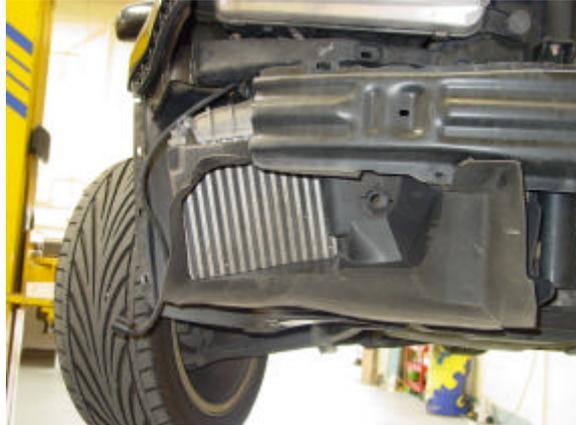
9/ Disconnect the upper and lower hose connections to the stock intercooler by using a flat blade screwdriver to dislodge the clip that locks into place on the hose coupling.
