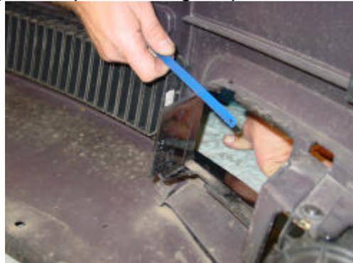
21/ Refit the bumper cover remembering to reconnect the fog light connections and also the ambient temp sensor connector. Refit all required parts in reverse order of removal. Remove all tools, axle stands and Jacks.
