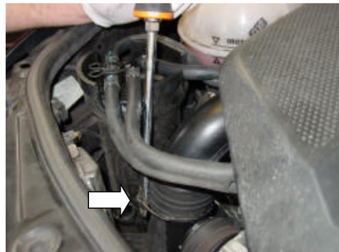
13/ Remove the 2 radiator air deflectors. There is one each side of the radiator fastened with one T25 Torx screw.
