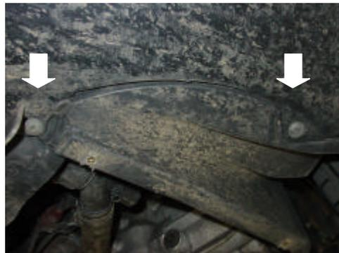
4/ Press in the centres of the 3 x plastic trim clips at the bottom front edge of the bumper. Then prize away the outer using a flat screwdriver or a trim pry tool. Retrieve the centres once the bumper has been completely removed.
