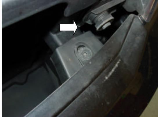
6/ Now pull outwards both side fixings of the bumper as shown.
