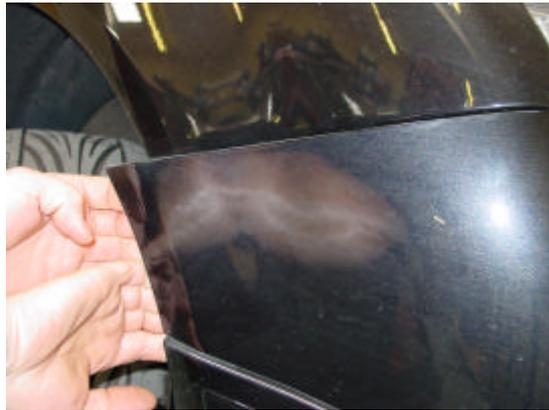
7/ The bumper cover can now be pulled forward and the fog light and ambient temp sensor plugs can be disconnected. The complete bumper can now be removed from the vehicle.
