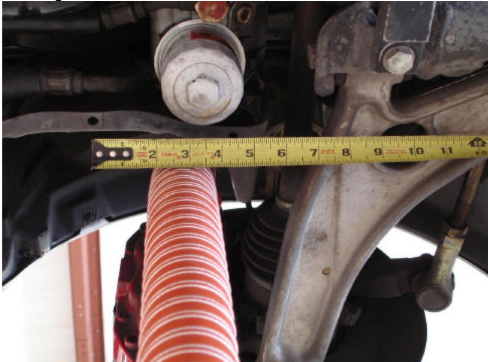
While routing the ducting, be sure to use the supplied Zip/Cable ties to secure the ducting to solid points within the engine bay (such as to the undertray) and also to the front bumper away from any moving parts and in such a way that vibrations will not cause rubbing that will damage the ducting.
