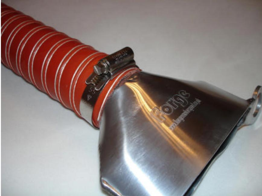
**\* Note:** Please ensure that the drive mechanism of the clamp (screw) is positioned on the logo side of the caliper duct facing the front of the car when tightening it down around the ducting. This is necessary to ensure proper clearance between the clamp and the drive shaft when the wheel is turned in. If the screw of the clamp is facing rearwards, damage may occur to the driveshaft and/or clamp.
