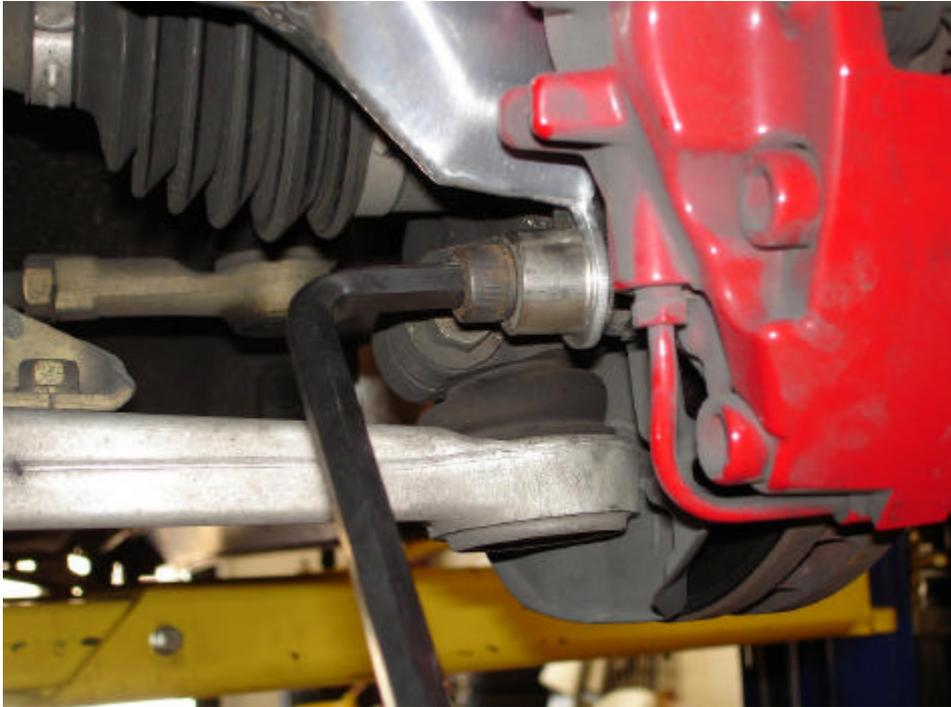
Once installed, this is how the caliper duct should look:
