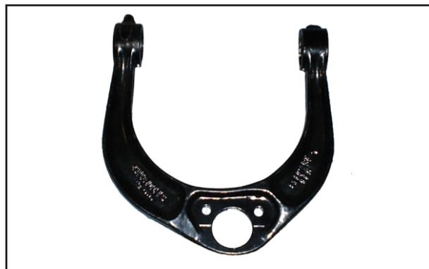
Photo 1. Cast arm with bushes removed.
