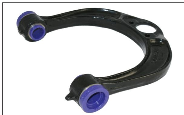
Photo 3. Cast arm with outer shells and bushes installed.
