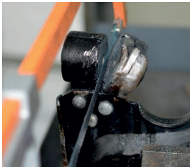
Cut original bush shoulder to enable it to be pressed out.
