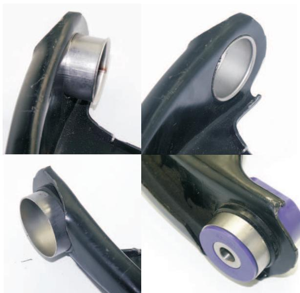
Fig 2: Fitting shell and fitted bush
